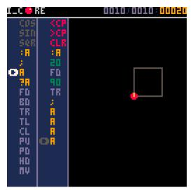
When a sequence of instructions needs to be repeated, a name can be associated to it (A, B or C). The set of instructions begins with the prefix :A, :B or :C. The character; ends the set. The letters A, B and C execute the set (declared with :A, :B or :C). The length of the script to draw the square can be optimized... but it costs more execute steps (20 \iff 14).
