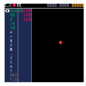
I\_CORE statistics are displayed on the upper right of the screen. The violet numbers oooo:oooo indicates the current line number and the number of lines of the current script. The orange one shows the number of execution steps needed to terminate the script.
